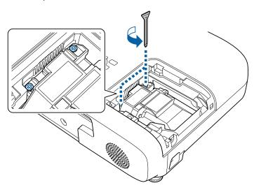
**6** Grip the raised section of the lamp and remove it.
