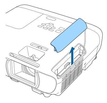
**3** Pull the air filter out of the projector.
