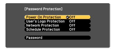
If you do not see this menu, hold down the [Freeze] button on the remote control for 5 seconds until the menu appears.
