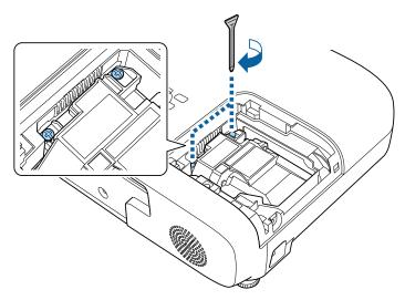
**9** Replace the lamp cover and tighten the screw to secure it.
