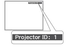
While holding the [ID] button, press the number button that matches the ID of the projector you want to operate.
