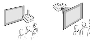
Make sure you select the correct **Projection** option in the projector's **Extended** menu according to the installation method being used.
