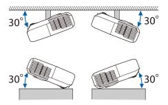
If you use the projector tilted at an angle of more than 30° it could be damaged and cause an accident.
