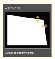
To reset the Quick Corner corrections, hold down [Esc] for about 2 seconds while the Quick Corner adjustment screen is displayed, and select Reset Quick Corner. Select Switch to H/ V-Keystone to switch the image shape correction method to H/V-Keystone.
