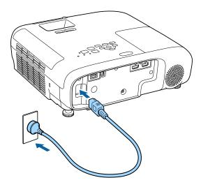
The projector's power indicator turns blue. This indicates that the projector is receiving power, but is not yet turned on (it is in standby mode).
