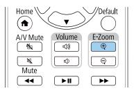
The projected image is enlarged focusing around the center of the image. You can enlarge the image between one to four times in 25 incremental steps.
