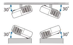
If you use the projector tilted at an angle of more than 30° it could be damaged and cause an accident.
