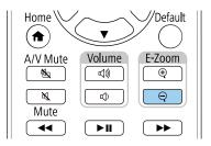
The projected image is reduced. You can reduce the image between 100% to 50% in incremental steps.
