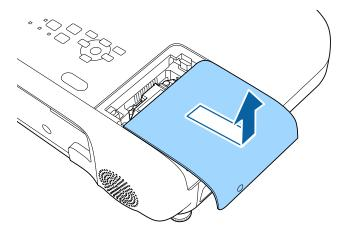
Loosen the screws securing the lamp to the projector. The screws do not come all the way out.
