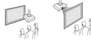
Make sure you select the correct **Projection** option in the projector's **Extended** menu according to the installation method being used.
